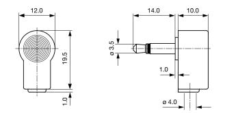
Cable diameter max. 4.0 mm
