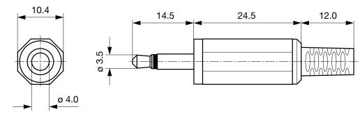
Cable diameter max. 4.0 mm
