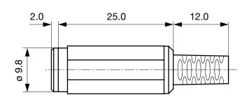
Cable diameter max. 4.0 mm
